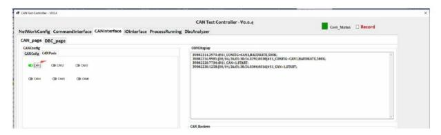
When there is data on the CAN line, the data on the CAN line will be displayed on the interface as shown below.
