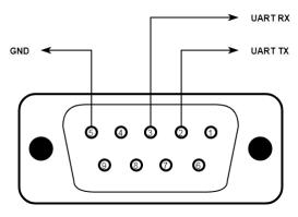
The SCU10 has one RS-232 port that can be used for the communication with the device. The default parameters of the UART are the following:
